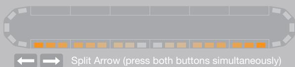
Pressing the PATTERN button while in Right Arrow, Left Arrow or Lightbar Flash mode will cycle through the available patterns.
