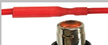
Apply heat thoroughly to the entire strip using hot air gun or similar tool.
