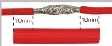
Cut length of heatshrink allowing for approximately 10mm of overlap.
