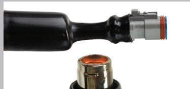
Apply heat starting at the connector end.
